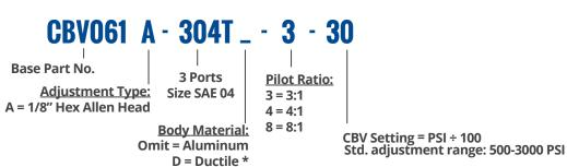
Not all Pilot ratios are available from stock. 3:1 ratio is the standard offering. \*Ductile bodies have limited availability. Ductile bodies are recommended for working pressures over 3000 PSI.
