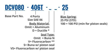
\* Ductile bodies have limited availability. Ductile bodies are recommended for working pressures over 3000 PSI. \*\* Fluorocarbon seals are used when temperatures exceed 212  $^{\circ}$  F (100 $^{\circ}$  C).
